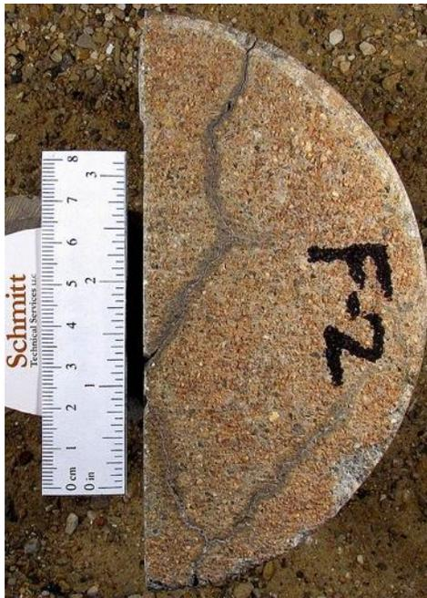
(a) Core top/wearing surface. Scale is in inches and centimeters.
