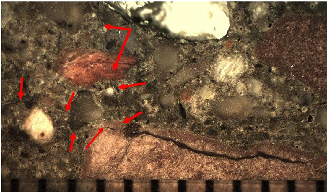
Figure 23. Magnified lapped slice of Core G1 showing cracks radiating out from a rimmed, dolomite coarse aggregate particle (red arrows). White, brucite (and other related) deposits line the cracks and voids. This is typical of damage due to alkali-carbonate reaction. Scale is in millimeters.
