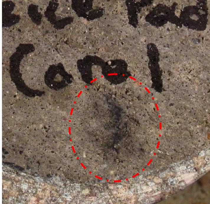
Figure 5. Close-up of the wearing surface in Core 1 (De-Ice Pad). Within the red dashed circle is an area of minor surface pitting.
