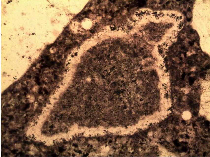
Figure 9. Thin section photomicrograph of a rimmed chert particle in Core C7. Vertical field of view is 1.1 mm. Plane polarized light.
