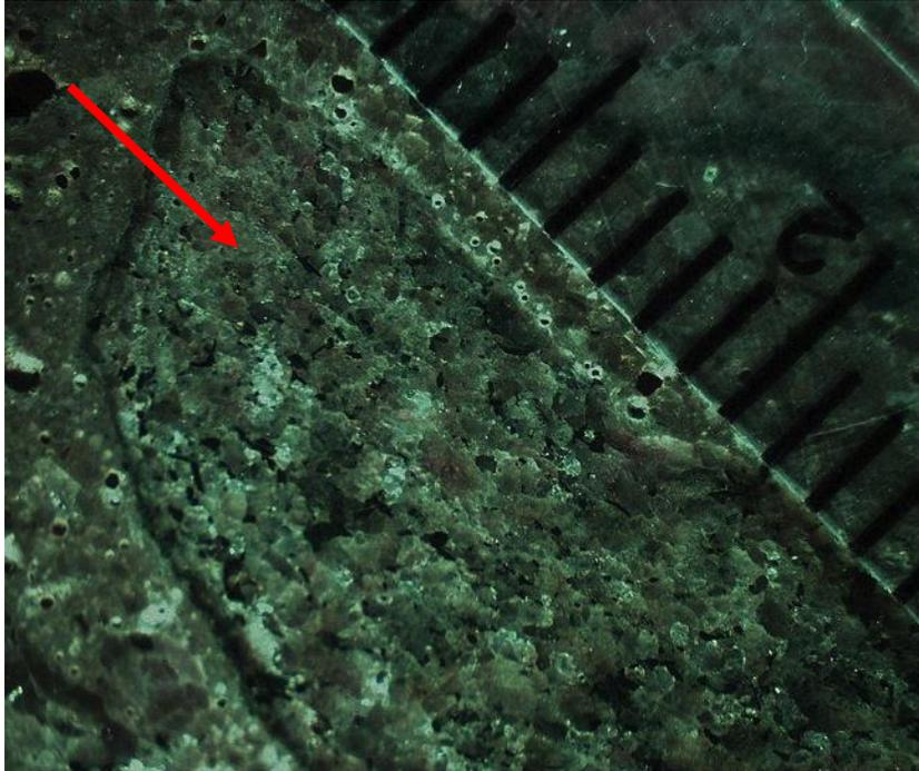
Figure 9. Photomicrograph of Core B-1 illustrating a rimmed gneiss particle (red arrow). Scale is in millimeters.
