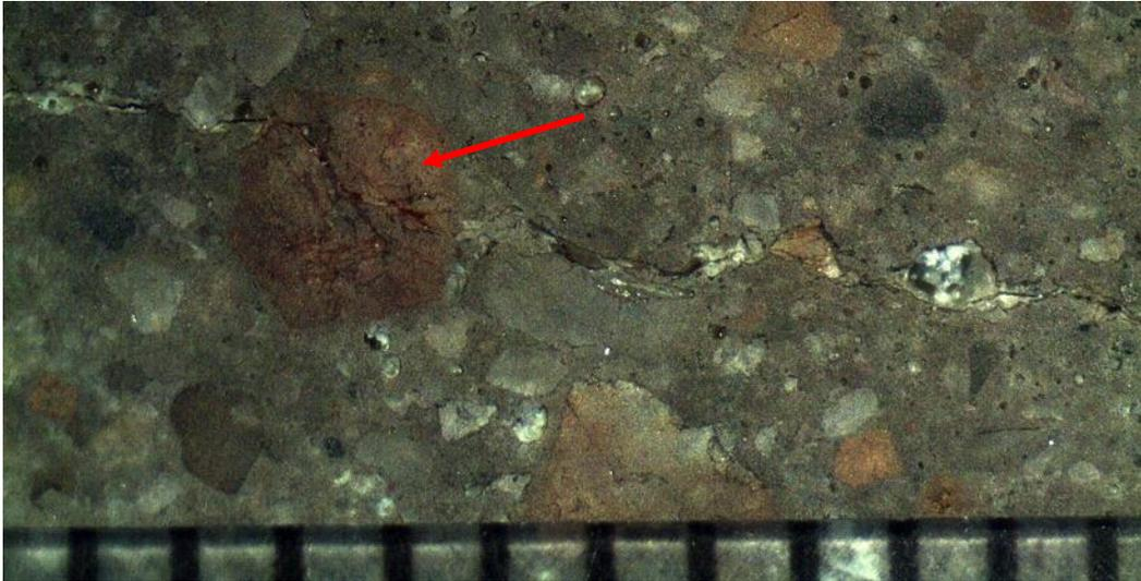
Figure 5. Lapped surface of Core C1 showing horizontal oriented cracking and microcracking extending outward from a metaquartzite fine aggregate particle (red arrow). Scale is in millimeters.
