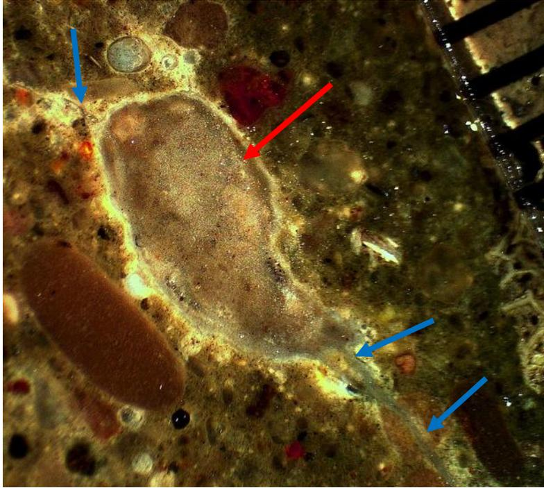
Figure 9. Photomicrograph of Core 9 illustrating a crack radiating from a rimmed chert particle (red arrow) into adjacent paste. The crack is filled with white alkali-silica gel (blue arrows). Scale is in millimeters.
