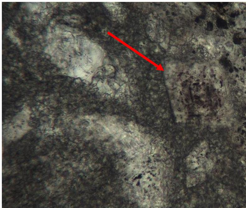
Figure 6. Thin section photomicrograph of Core 1 illustrating dolomite rhomb with an argillaceous inner core and non-argillaceous outer rim and ragged upper crystal face (red arrow). 120X magnification. Vertical field of view is 0.7 mm. Plane-polarized light.
