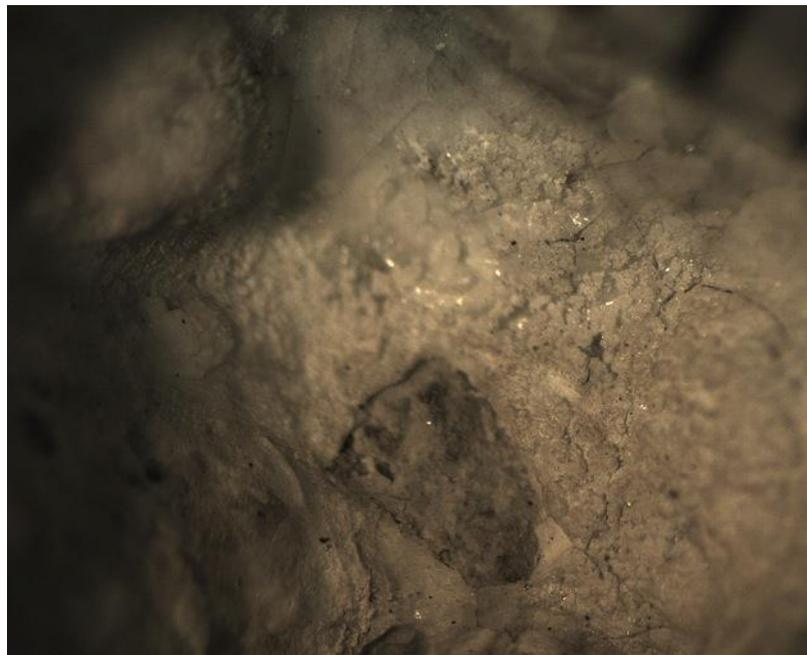
Figure 25. Void lining in Core G1 containing various, secondary deposits, including white, pearly brucite; translucent magnesite; dull, white, botryoidal clusters of nesquehonite; amorphous, desiccated (and pattern cracked) alkali gel (and other related) deposits. Scale is in millimeters.
