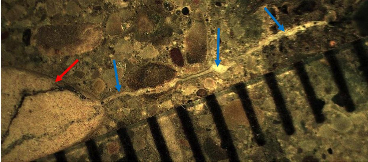
Figure 7. Lapped surface of Core 4 illustrating a crack radiating from a rimmed, beige chert particle (red arrow) into adjacent paste. The crack is filled with white alkali-silica gel (blue arrows). Scale is in millimeters.
