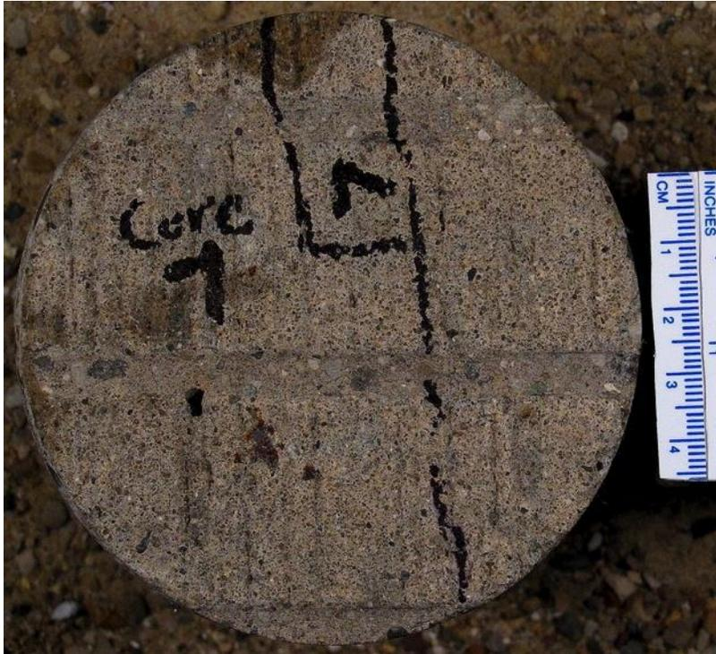
(a) Core top/wearing surface. Scale is in centimeters.
