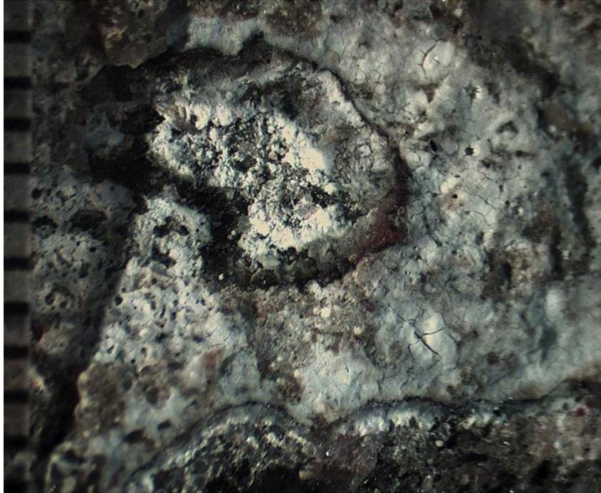
Figure 23. Photomicrograph of alkali-silica gel lining a crack in Core R-6. The reacting gneiss particles are delineated by red arrows. Scale is in millimeters.
