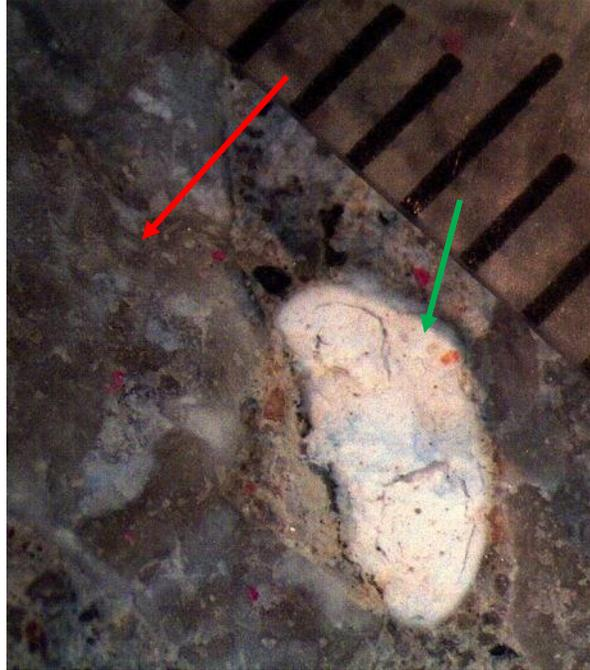
Figure 3. Photomicrograph along a freshly fractured surface of Core D8. Red arrow points to a reacting chert coarse aggregate particle with an alkali-silica gel filled void (green arrow) adjacent to the reacting particle. Scale is in millimeters.
