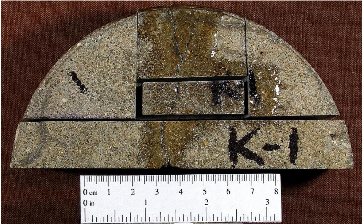
(b) Core top/wearing surface. Scale is in centimeters.
