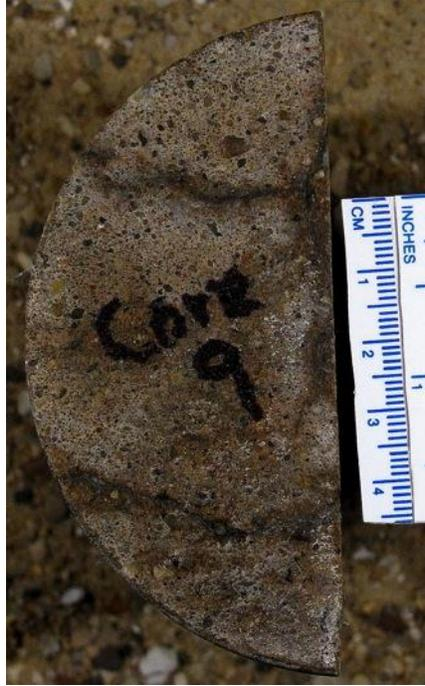
(a) Core top/wearing surface. Scale is in centimeters.
