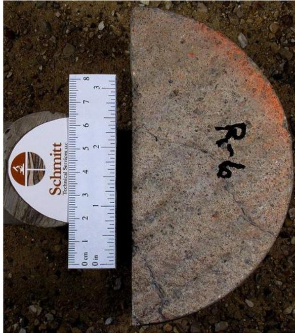
(a) Core top/wearing surface. Scale is in centimeters.
