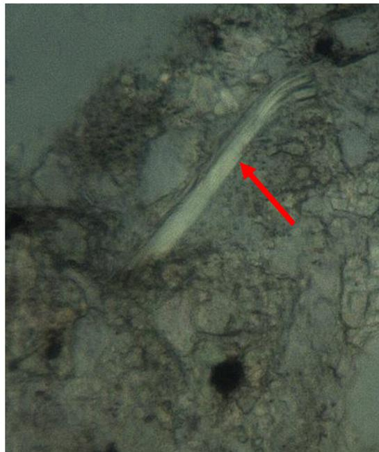
Figure 15. Thin section photomicrograph of Echo 5 – Core 4 showing coarse, fibrous brucite (red arrow) within a dolomite coarse aggregate particle. Vertical field of view is 0.25 mm. Plane-polarized light.
