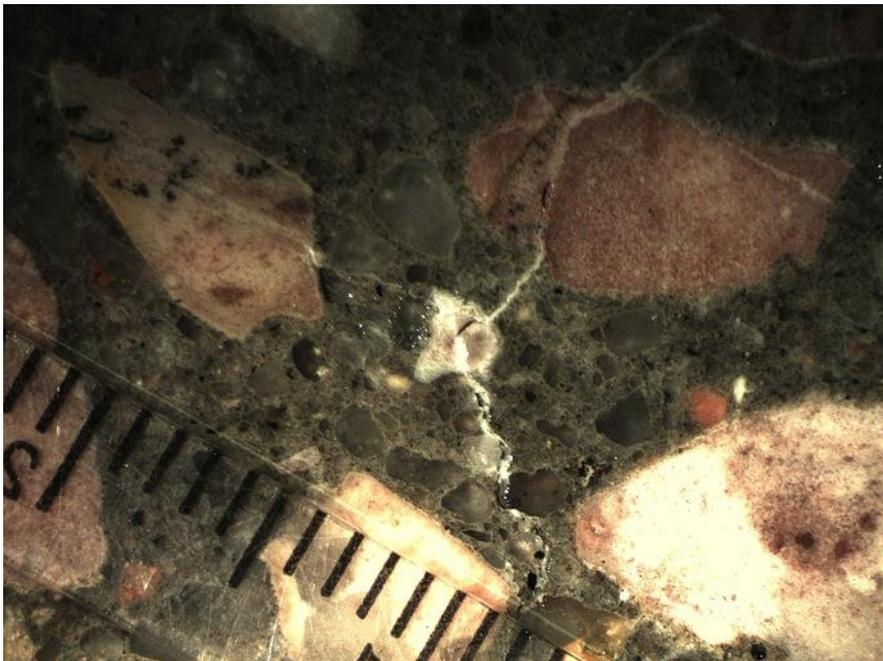
Figure 8. Photomicrograph of the magnified lapped slice of Echo 5 – Core 4 showing cracks radiating out from a small, dolomite coarse aggregate particle. White, brucite (and other related) deposits line the cracks. This is typical of damage due to alkali-carbonate reaction. Scale is in millimeters.
