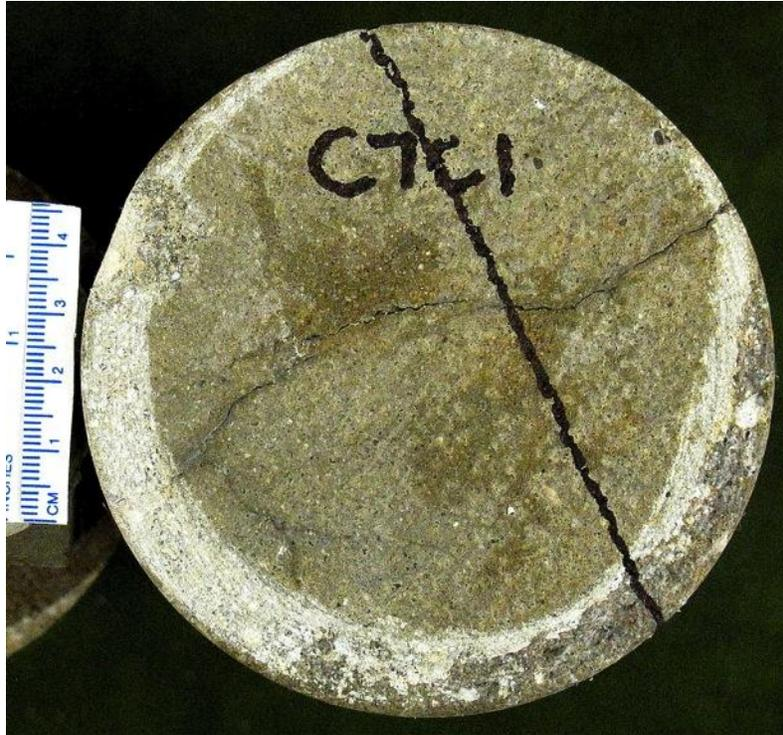
(a) Core top/wearing surface. Scale is in centimeters.
