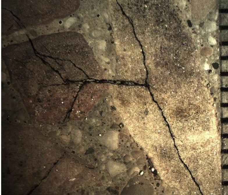
Figure 20. Magnified lapped slice of Core C1C7 showing cracks radiating out from reacting dolomite coarse aggregate particles. White, brucite (and other related) deposits line the cracks and voids. This is typical of damage due to alkali-carbonate reaction. Scale is in millimeters.
