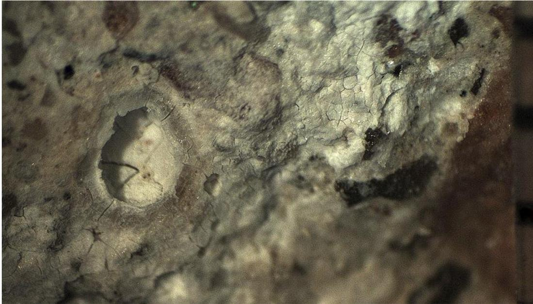
Figure 22. Crack surface in Core C1C7 lined with various, secondary deposits, including white, pearly brucite; translucent magnesite; amorphous, desiccated (and pattern cracked) alkali gel (and other related) deposits. Scale is in millimeters.
