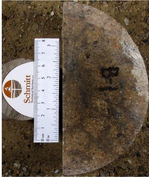
(c) Core top/wearing surface. Scale is in inches and centimeters.
