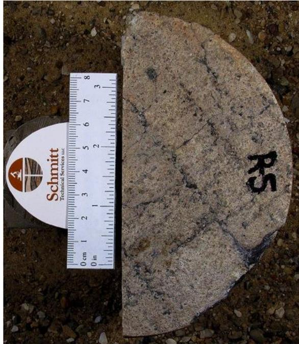
(a) Core top/wearing surface. Scale is in centimeters.
