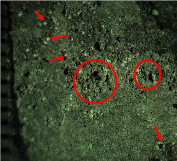
Figure 16. Photomicrograph of Core F-2 illustrating air-void clusters (within red circles) and ettringite filled voids (red arrows). Scale is in millimeters.
