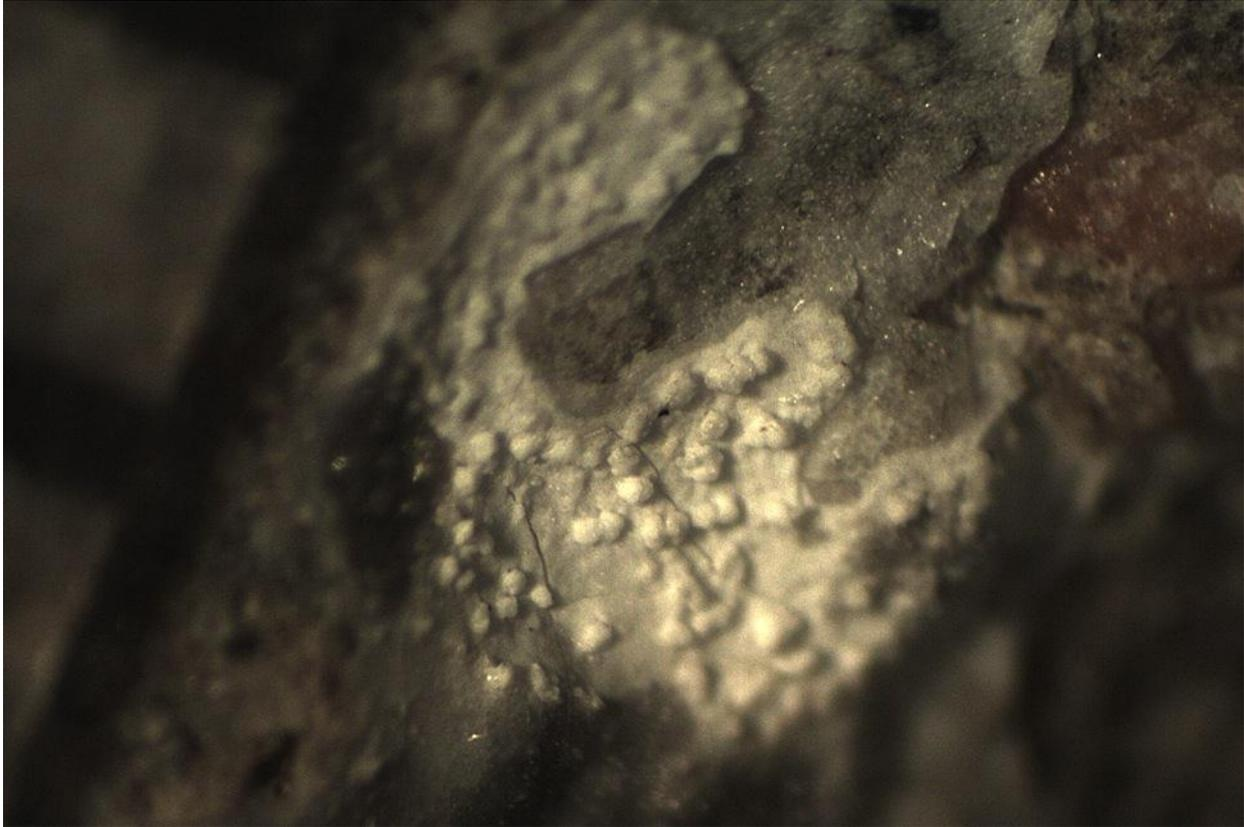
Figure 26. Crack surface in Core G1 lined with various, secondary deposits, including white, pearly brucite; translucent magnesite; and dull, white, botryoidal clusters of nesquehonite. Scale is in millimeters.
