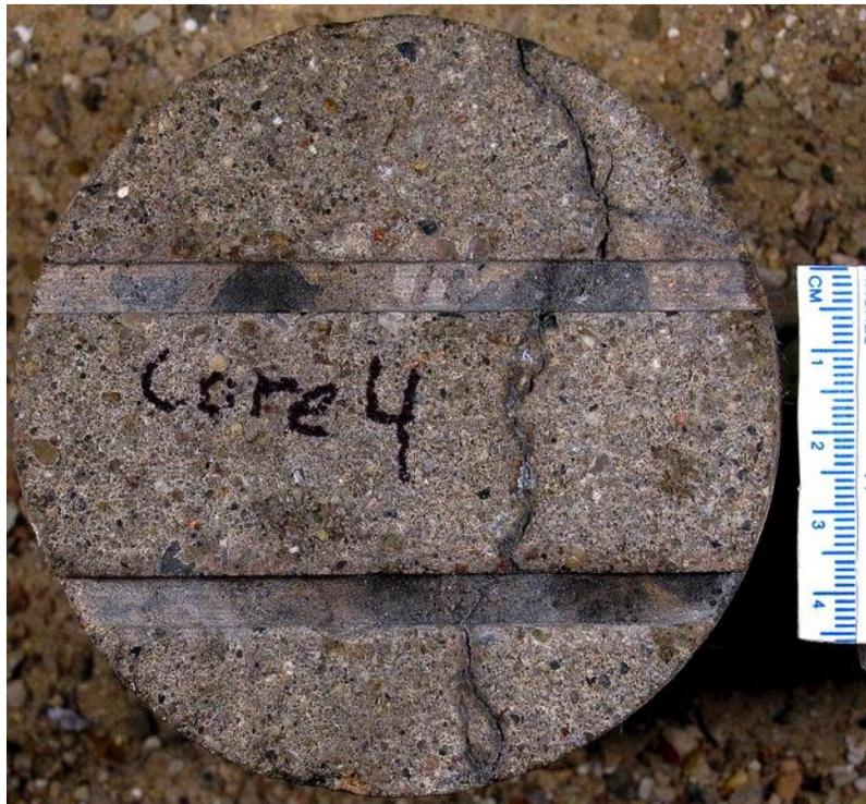
(b) Core top/wearing surface. Scale is in centimeters.
