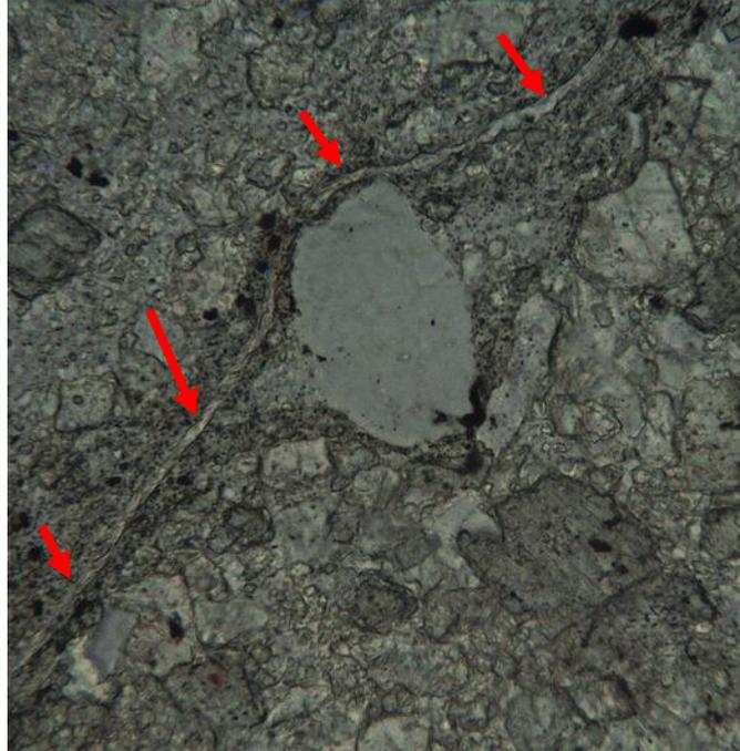
Figure 12. Thin section photomicrograph of Echo 5 – Core 4 illustrating a crack within a dolomite coarse aggregate particle (red arrows). The crack is lined with brucite and rock adjacent to the crack has been converted to a fine-grained calcite as compared to the coarser-grained dolomite further away from the crack. Vertical field of view is 0.60 mm. Plane-polarized light.
