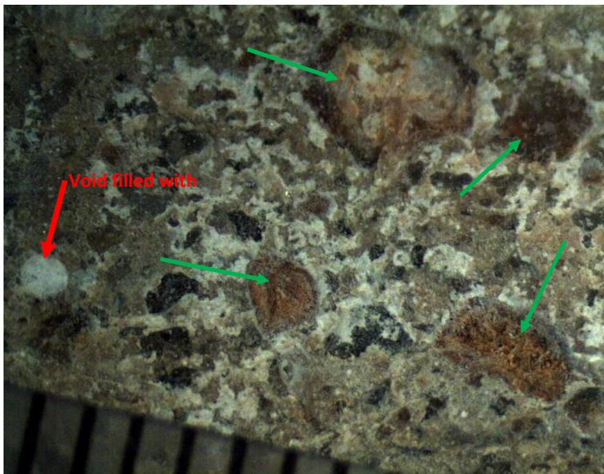
Figure 6. Magnified cracked surface in Core C1 where white alkali-silica gel lines the crack and voids adjacent to the crack. Several, cracked, rimmed and reacting chert and metaquartzite particles are present along the crack (green arrows). Scale is in millimeters.
